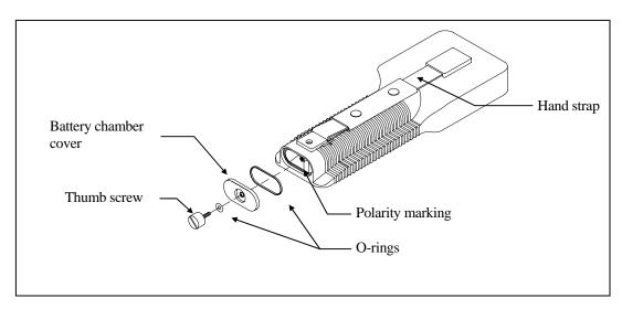
There is a small label inside each of the two battery-chamber sleeves. These labels illustrate the correct way to install the batteries into each sleeve of the battery-chamber.
